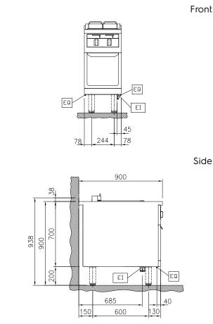
EI = Electrical inlet (power) EQ = Equipotential screw
